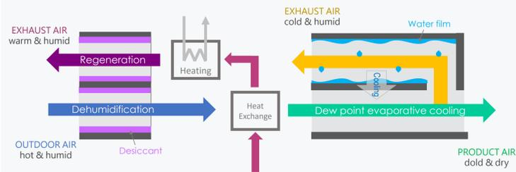
Independent desiccant dehumidification and dew point evaporative cooling.
