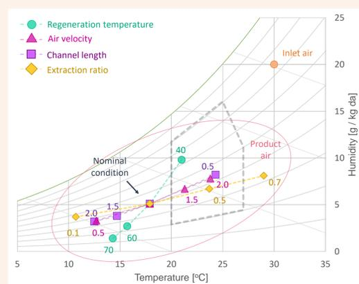
Effect of varying regeneration temperature, channel length, air velocity, and product air extraction ratio to product air minimum temperature & humidity in CoDECS.
