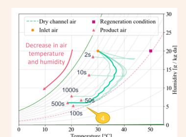
Psychrometric plot of dry air in CoDECS at nominal operating condition and at different time periods.
