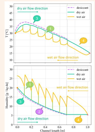
Temperature and humidity distribution along the dry and wet channels of CoDECS at nominal operating condition and  $t = 500s$ .
