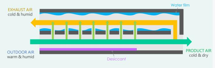
Combined desiccant dehumidification and dew point evaporative cooling system (CoDECS).
