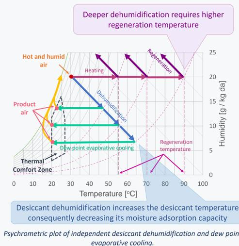
Psychrometric plot of independent desiccant dehumidification and dew point evaporative cooling.
